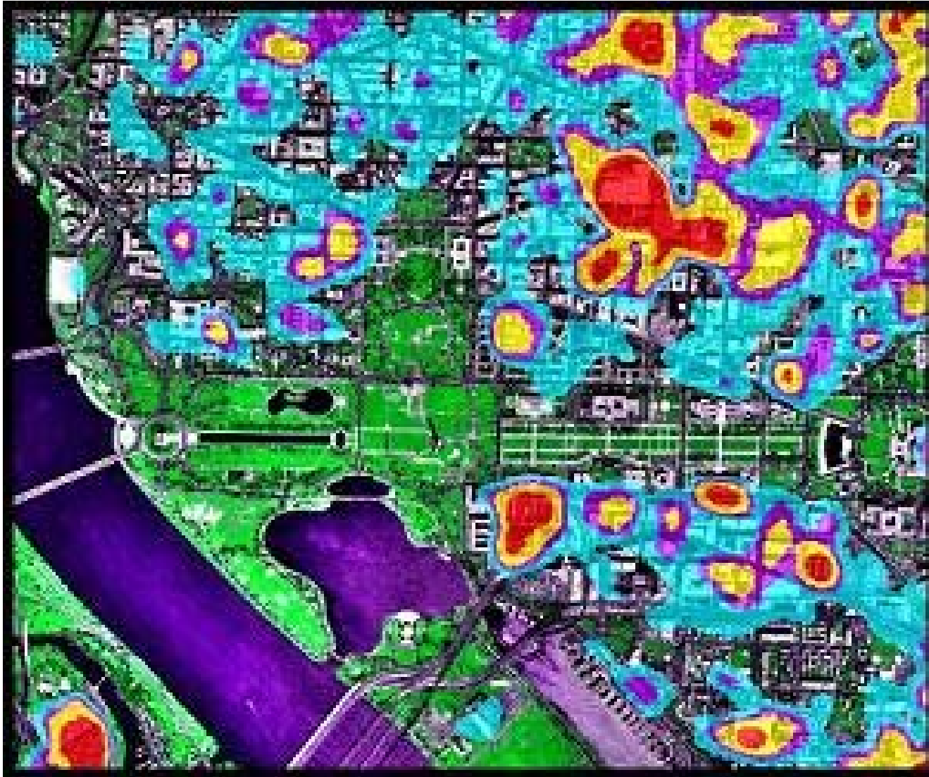
This is a thermally imaged map of Washington, D.C. showing its summer temperatures. Red is hot. Purple is cool.
