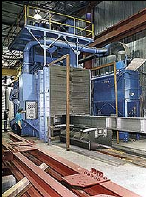
Shot blast cleaning with the use of abrasives
