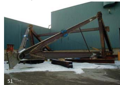
Fig. 2.1A A special physical mock-up was made for Pearson International Airport. Although minor modifications were made to the detailing for subsequent elements, it was incorporated into the project without any issue.
