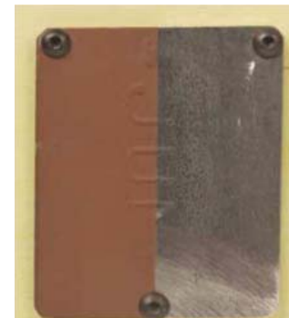
Fig. 3.1 Mill marks removed. Courtesy of AISC
