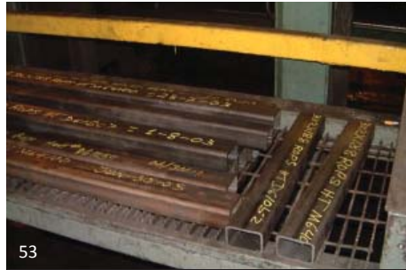
Fig. 2.2 One half standard fabrication tolerances are required for all elements to be incorporated into AESS 2 and higher.
