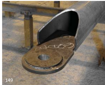
Several kinds of cuts are required to connect this plate to the HSS member. to create a pin connection.
