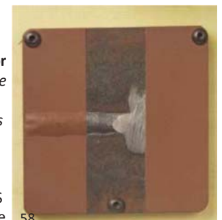
Fig. 3.2 Butt and plug welds ground smooth. Right side shows groove weld ground smooth. Courtesy of AISC
