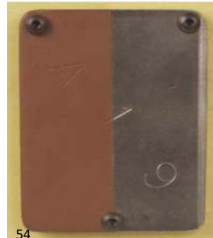
Fig. 2.3 Fabrication marks not apparent. Courtesy of AISC
