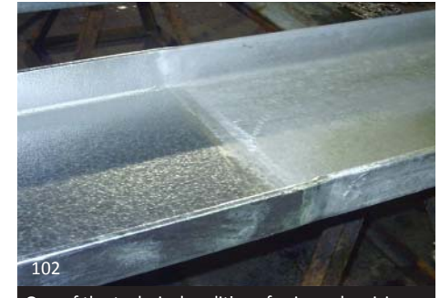
One of the technical realities of using galvanizing as a "finish" lies in the inconsistency of the product. The difference in this photo is due to finishing temperatures. If galvanizing is used as a final coating on an AESS project differentials in finish must be both understood and detailed into the project.
