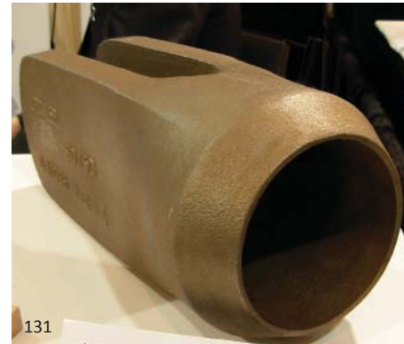
This is a cast connector that would form the end condition of a round HSS section or pipe. You can see the “orange peel” like finish of the raw casting.
