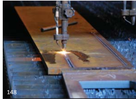
Automated torch cutting a piece of steel plate. If torch cutting is used on AESS material the edges will need treatment to make them smooth and assist with even finish applications.
