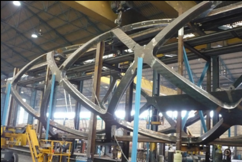
Images of the steel fabrication. All custom sections whose curvature was created via brake forming. Welds all ground smooth. AESS4
