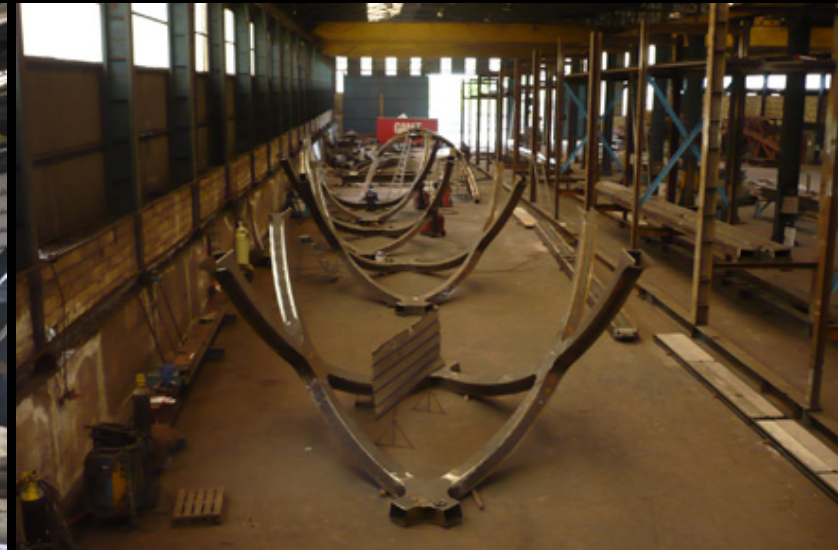
Images of the steel fabrication. All custom sections whose curvature was created via brake forming. Welds all ground smooth. AESS4
