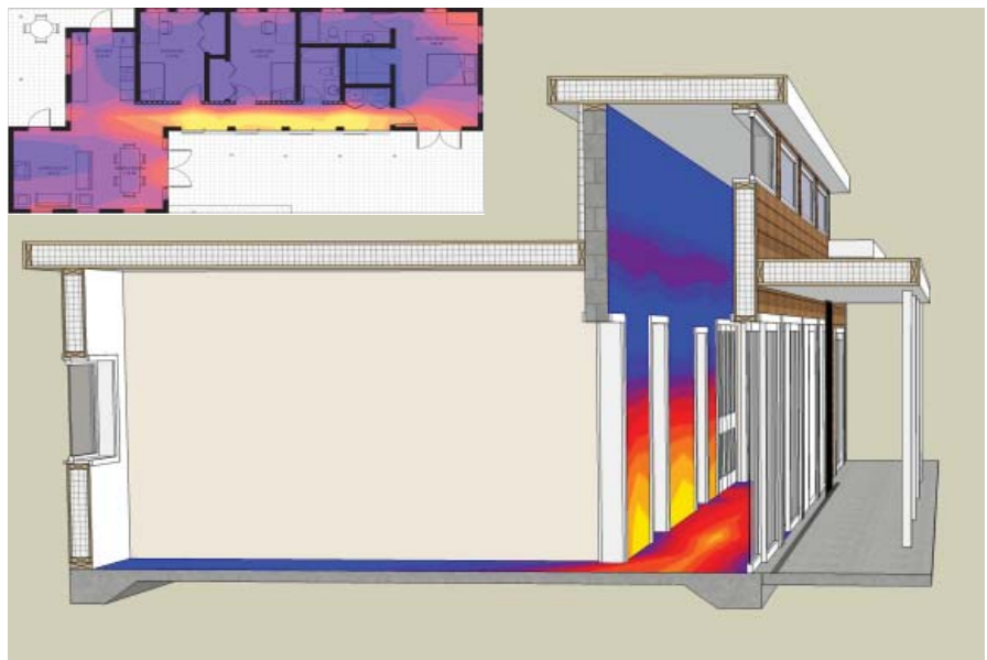
Fig 4: Design of a residential direct gain system with summer shading
