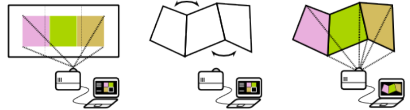
fig 6. diagram explanation of projection mapping
